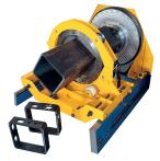
In addition to flat-bed cutting, MSF can be equipped with a cutting zone for round pipes and hollow profiles. Depending on type of the cutting zone, pipe diameters can reach from 020 mm to 0500 mm, hollow profiles cross-section from  $20 \times 20 \text{ mm}$  to  $300 \times 300 \text{ mm}$  at a max. pipe / profile length 6 m
