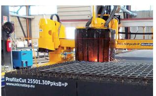
Laser scanner with independent Z, A and B axis for scanning shape and position of the profiles
