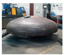
Full range of sheet as well as wide sizes of dome cutting application
