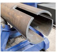
Area for cutting pipes, square and rectangular profiles equipped with rotary pipe positioner
