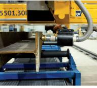
Cutting of structural profiles as I,H,U and L in separate area
